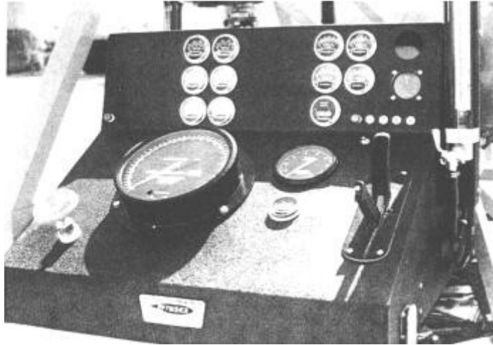
Dyno test stand used for RotorWay engine development, air show demonstrations, and production engine run-ins.
